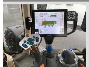
Due to the compatibility of the Strautmann ISOBUS control (ISOBUS AEF certification), most varied terminals can be used for the Strautmann forage wagons. Thus, depending on the tractor type, all machine functions can be operated via the tractor joystick.
